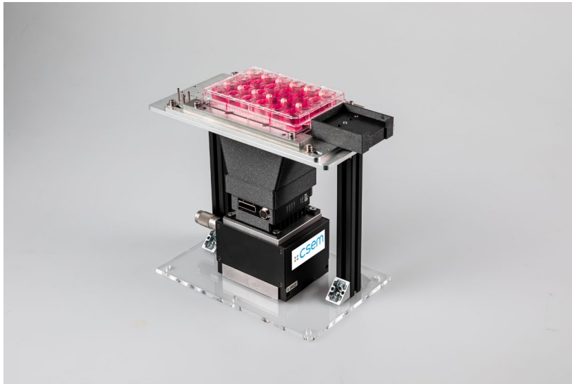
First prototype of the optical reading module for contractility measurement. Image: CSEM.
